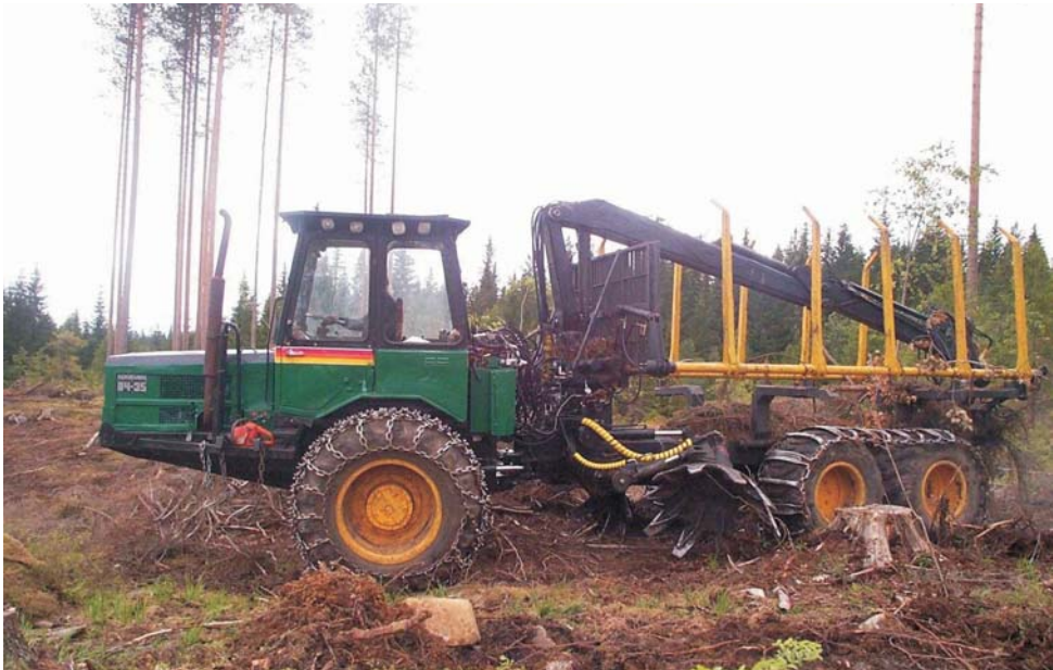
Figure 35. A forwarder equipped with an enlarging load space for off-road transport of logging residues and with a disc scarifier for simultaneous site preparation. A prototype constructed by Antti Varis (Courtesy of the Forest Centre of North Karelia).
