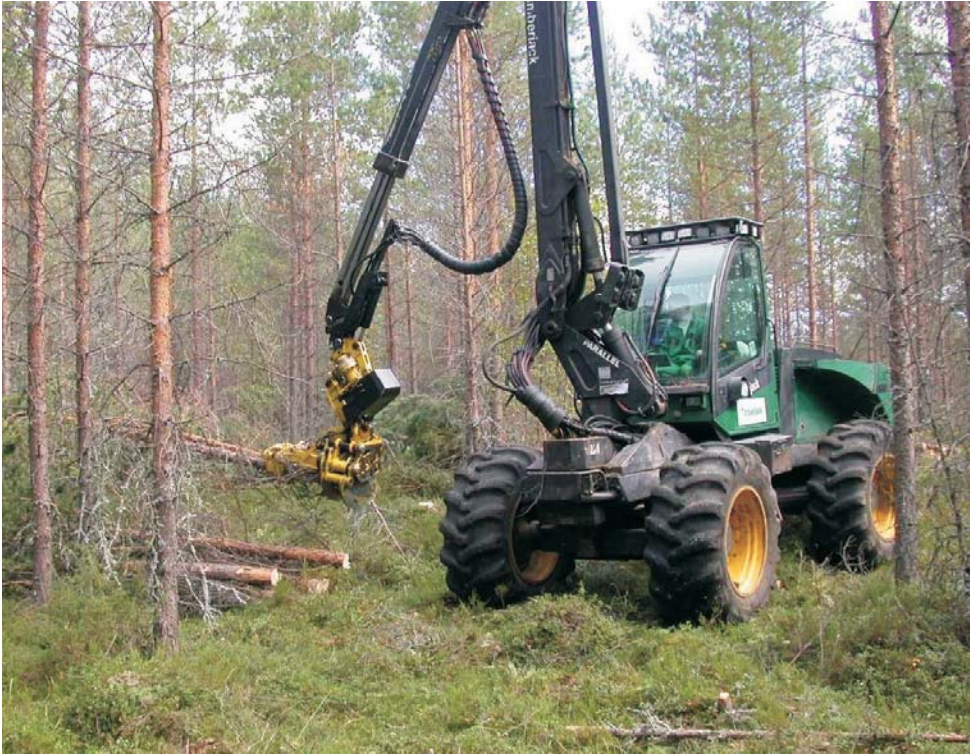
Figure 34. Timberjack 770 harvester equipped with the accumulating Timberjack 730 feller head for small-tree operations (Courtesy of Timberjack Oy).
