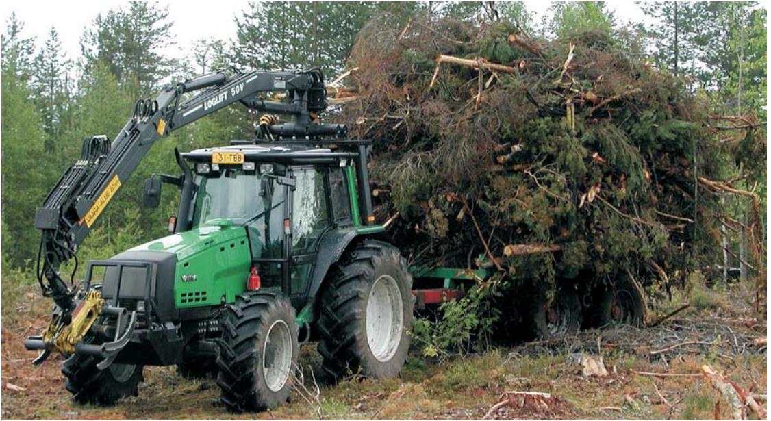
Figure 21. A Valtra farm tractor-based residue forwarder with enlargening load space (Courtesy of TTS-Institute).
