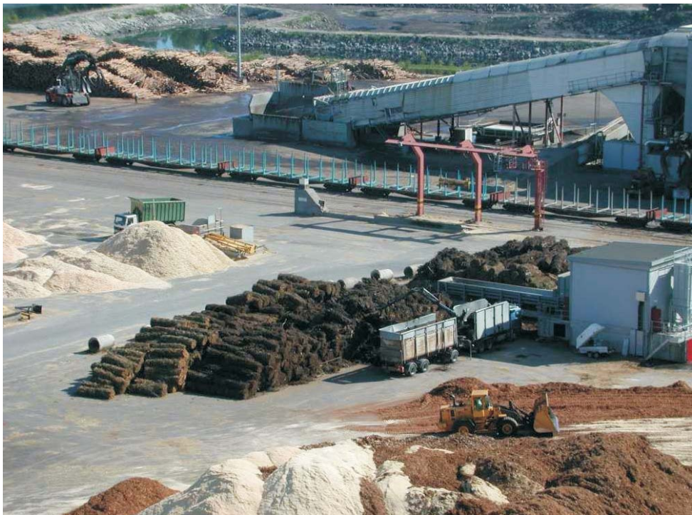
Figure 12. A view of the wood fuel yard of the 550 MW th Alholmens Kraft CHP plant. Receiving and crushing station for CRL bundles on the right side. Pulpwood piles on the background (Courtesy of E.V.A.).
