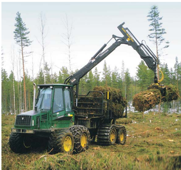
Figure 20. Off-road transport of residue bundles with a conventional forwarder (Courtesy of Timberjack Oy).
