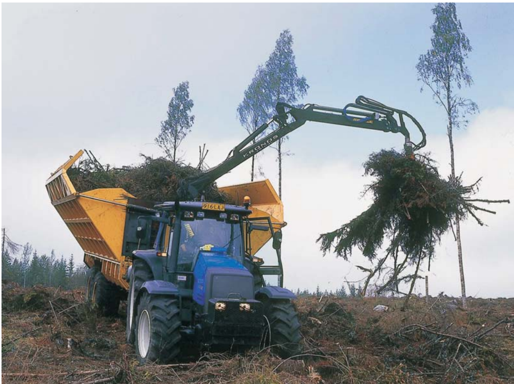
Figure 22. The load-compacting HavuHukka forwarder for transporting residues from logging site to satellite terminal (Courtesy of Vapo Oy).
